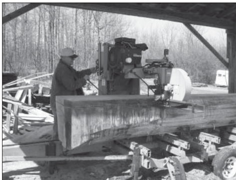
George Bowdish cutting the rudder from donated oak
